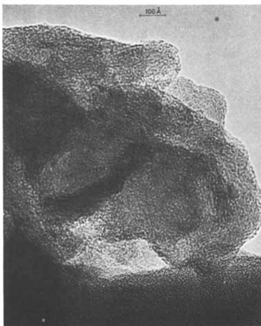
Figure 12. TEM of hard coke skin from uncoated Incoloy 800 tube.
